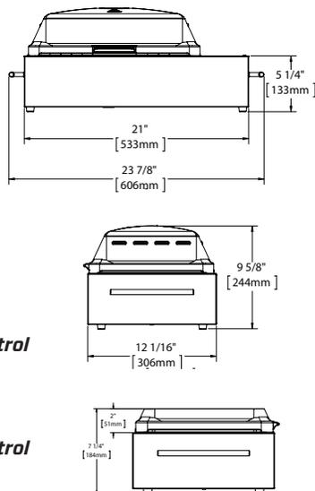
Introducing the patented SilKEN® Grill, a flameless and smokeless electric grill that incorporates a patent pending high temperature silicone lid. Ideal for all grill applications, the lid can collapse accordion-style to a height of two inches making it easier to tuck away in any convenient location. The lid has two handles, one on top and one on the front edge, and vents on three sides.
